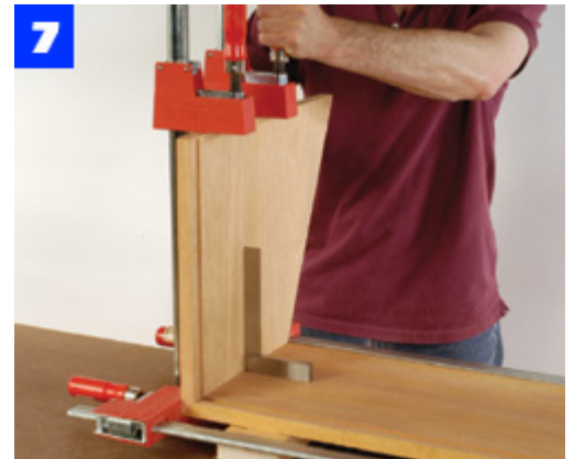
Apply glue and clamp the sides to the top. Clamp in both directions and check that the assembly is square.
