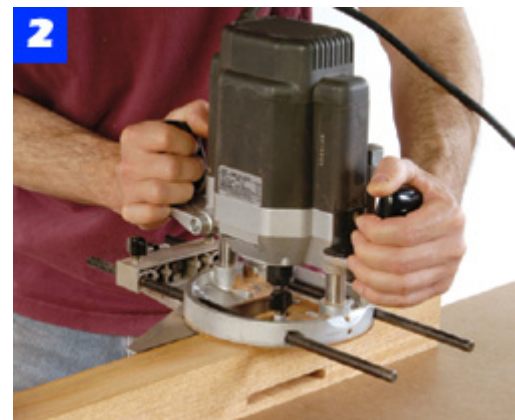
Lay out the mortise locations and use a router and edge guide to cut the mortises. Square the ends with a chisel.
