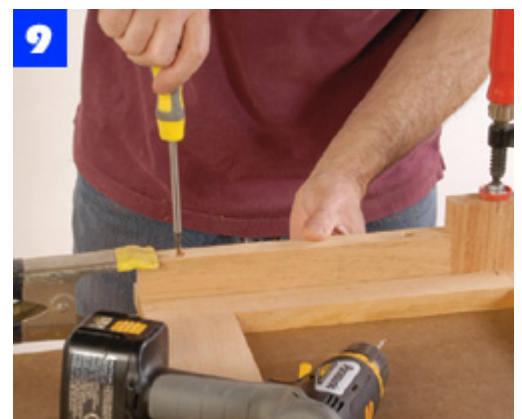
Join the frame dividers to the bottom drawer frame with joining plates. Secure the drawer guides with screws.
