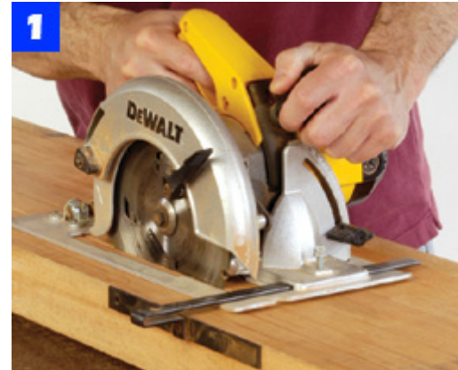
Use a circular saw to create the leg blanks. Cut halfway through the stock, then flip it over to complete the cut.
