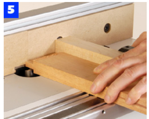
Cut all of the tenons with a router table and miter gauge. Use scrap stock behind the work to prevent splintering.
