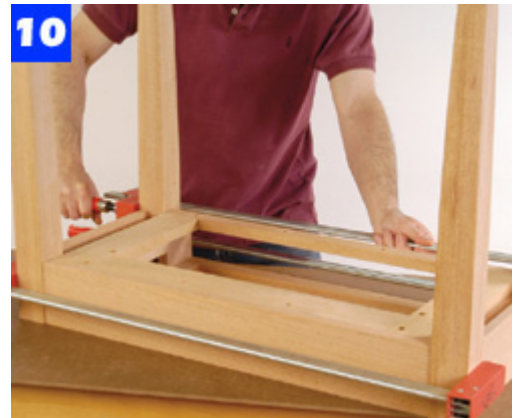
10 Join the side-rail/leg assemblies to the drawer-frame/rear-rail assembly. Use clamps to pull the joints tight.
