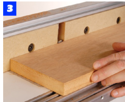
Shim the outfeed fence of a router table so it's aligned with the bit, and use your table to joint the stock edges.
