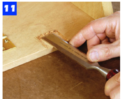
11 Lay out the hinge mortise locations on the case bottom and door. Use a sharp chisel to cut the mortises.
