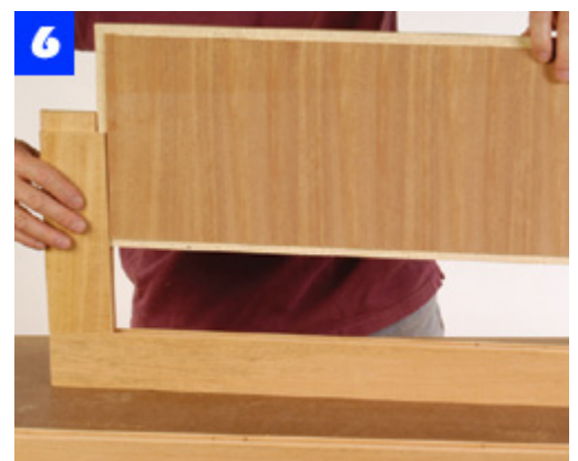
Assemble the back-panel rail and stiles, then slide the panel in its groove and add the remaining rail.
